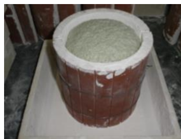
電気炉で焼成・発泡 Firing and foaming in an electric furnace
