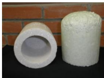
脱型後、内部加工 Internal processing after demolding
