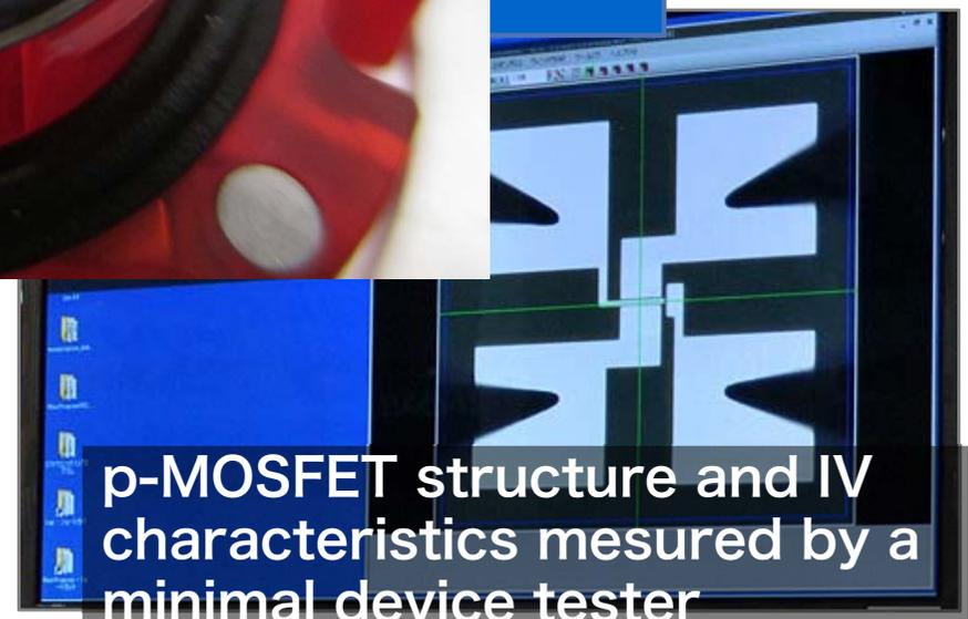
p-MOSFET structure and IV characteristics measured by a minimal device tester
